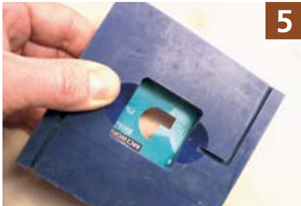
Place the die on an extruder die to check the fit.
