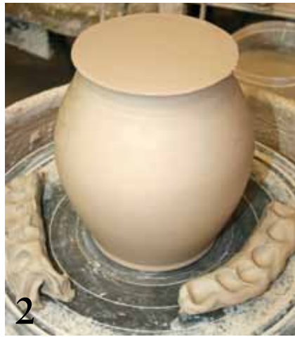
2 Cut the vase from the bat, flip it over and center it on the wheelhead.
