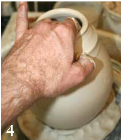
4 Cut a hole in the bottom, throw to widen it, then throw the wall to thin the clay.
