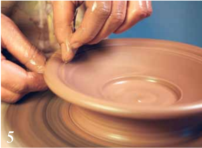
Compress the lip using a piece of plastic or chamois.
