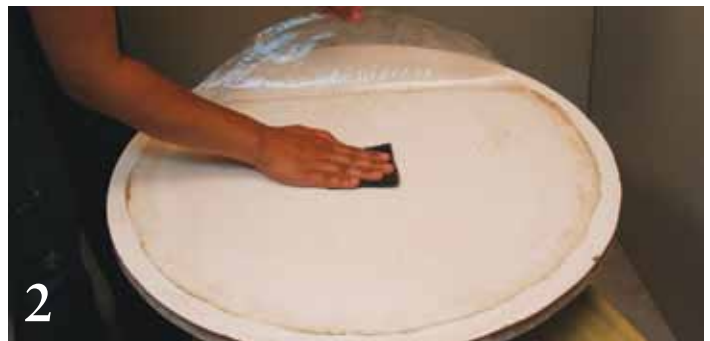
2 Dampen a large bat and smooth the cutout shower curtain on top of the bat.
