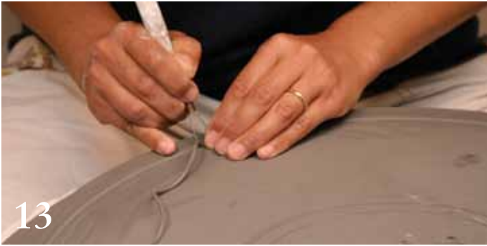
Trim the outside of the foot ring, mark the interior support ring, then trim away the clay between the two rings.
