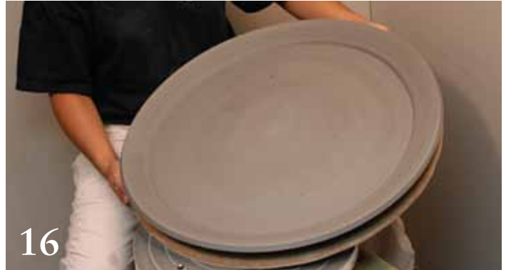
Carefully flip the plate back onto a clean, dry bat, and always transport it by carrying it as shown prior to firing to avoid warpage and cracking.
