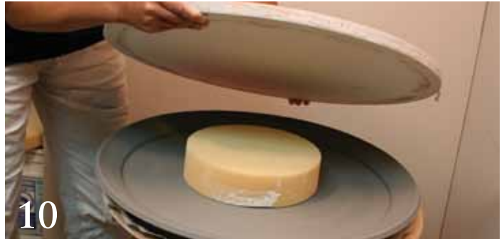
10 Place a foam sheet onto the center of the plate for support while flipping it over.
