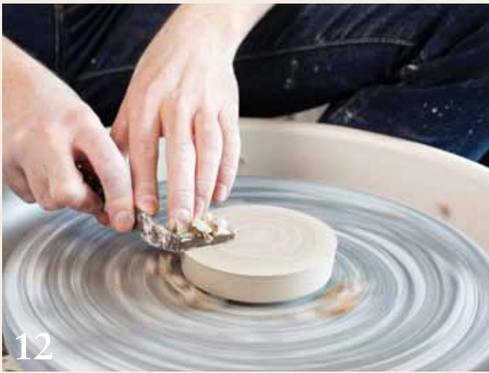
12 Trim excess clay from the top of the lid with a steel turning/trimming tool.
