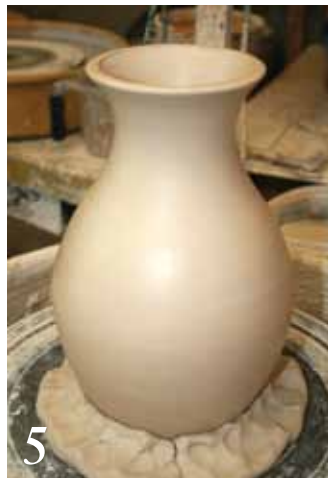
5 After thinning the wall, collar and refine the shape.
