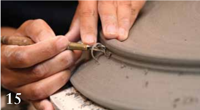
If you plan to hang the plate on the wall, carve a deep groove into the outside of the foot ring so you can wrap picture hanging wire around the foot after it's fired.
