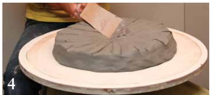
4 As the wheel spins, use a wooden paddle to further compress and flatten the mound until it's between 3–5 inches tall.
