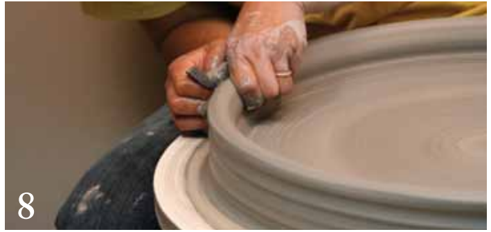
8 Pull the wall straight up using your index finger on the inside and a sponge and the knuckles of your other hand on the outside. Compress the rim after the pull.
