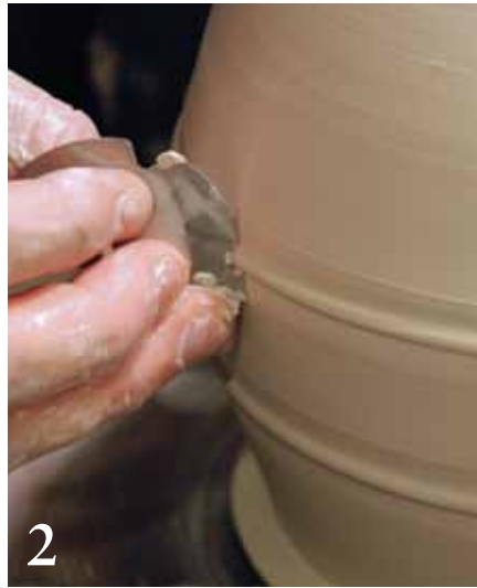
2 Using a modified rib, create horizontal decorative rings.
