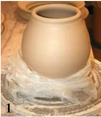
1 Throw a vase form, wrap the bottom in plastic, and dry the top to leather hard.
