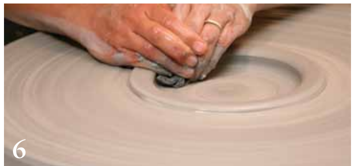
6 Wet your hands and hold a wet sponge in your dominant hand. Press down with both hands to open the form.
